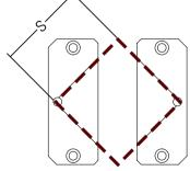
Circular Clamping Range (D): 1.87" - 3.15" Square Clamping Range (S): 1.87" - 3.15"
